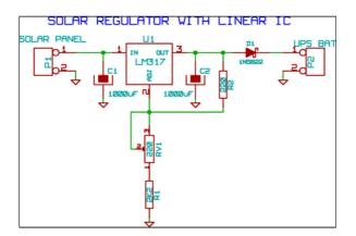
Figure 9. Charge regulator schematic
