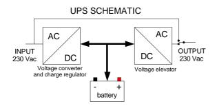
Figure 3. UPS internal schematic
