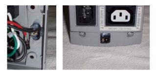
Figure 7. External recharge connector
