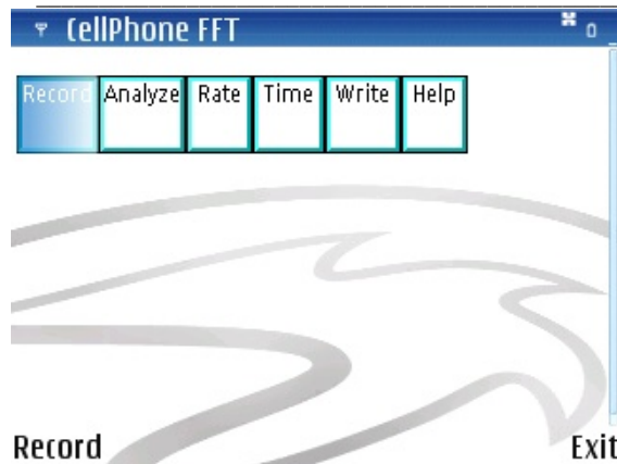
Figure 2. Menu options, Record a sound, Analyze recording, Time and Rate are parameters for data collection, and Write sound data to cell phone file.
