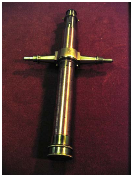
Figure 4 The telescope of a goniometer (F 539)
