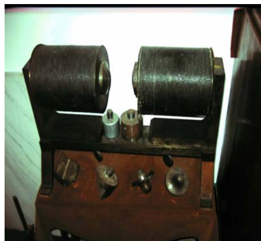
Figure 7. The electromagnet (G 843) used in FARADAY's experiment to study the rotation of the polarization plane. Also, pole heads for other uses.
