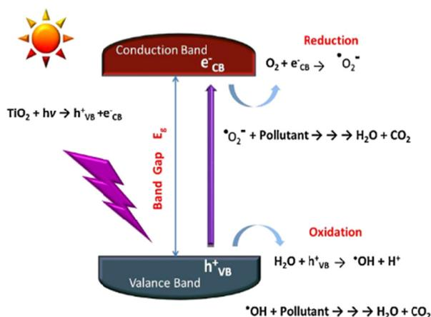
**Figure 1. Schematic illustration of several processes that occur after photoexcitation of pure TiO<sub>2</sub> with UV light [4]**
