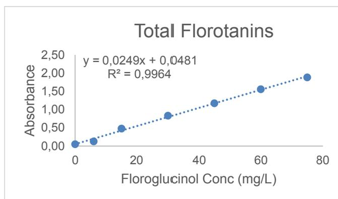
Figure 11. Calibration curve for the determination of total phenolics
