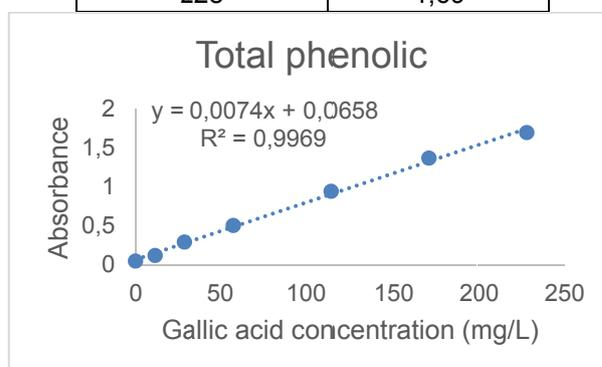
Figure 9. Calibration curve for the determination of total phenolics
