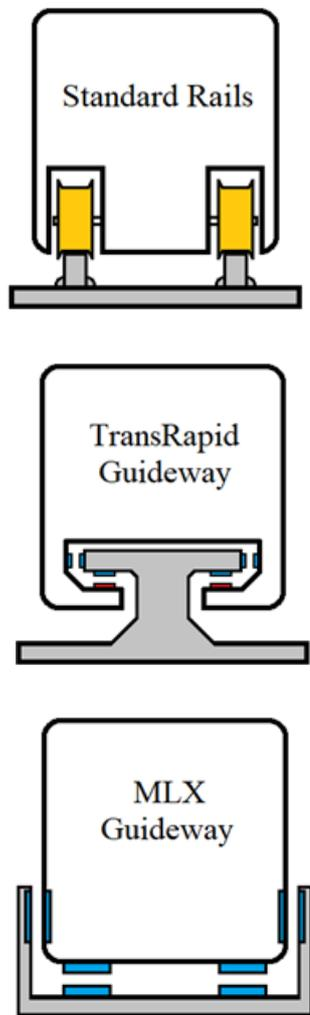
**Figure 2. Comparison of Wheel-Rail versus Guideways**
