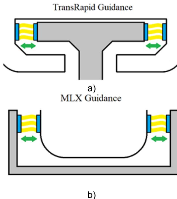
Figure 6. Guidance system of TransRapid and MLX (both use repulsive magnets)
