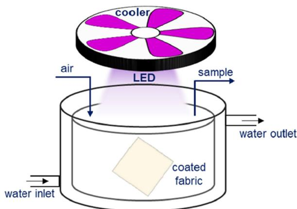
**Figure 2. Configuration used in photocatalytic experiments [1]**
