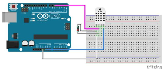
**Figure 4. Circuit for temperature and humidity measurements**
