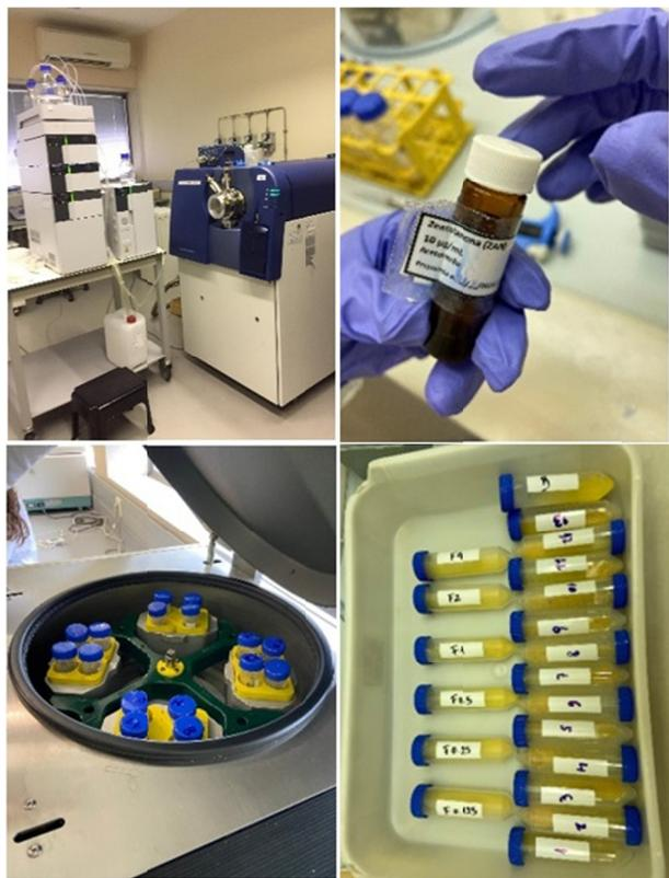
**Figure 1. Ultra-High-Performance Liquid Chromatography, internal standard (Zearaleone), maize centrifugation, and all samples**
