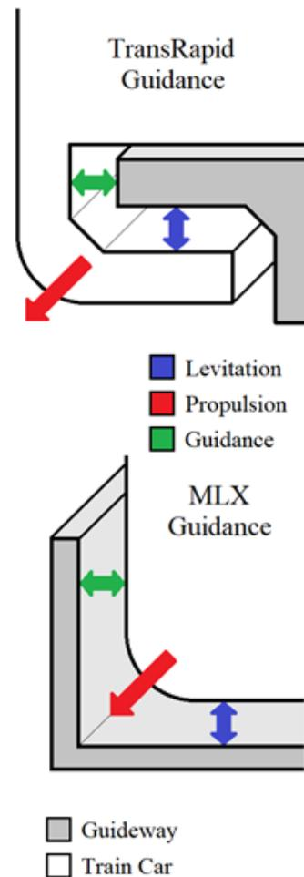
**Figure 3. Levitation, propulsion, and guidance in MagLev**
