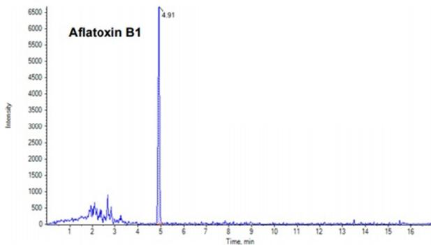
Figure 4. Chromatogram of a blank maize sample Aflatoxin FB1 (AFB1)
