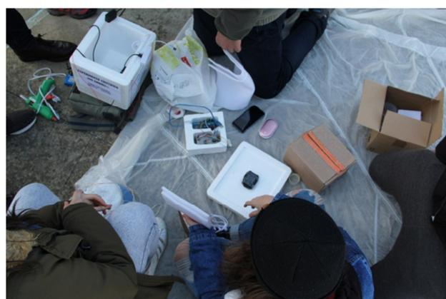
**Figure 5. Assembling the battery, heater and electronic systems in the payload box before launching**
