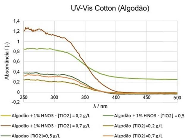
Figure 3. DRUV-Vis characterization of cotton substrates
