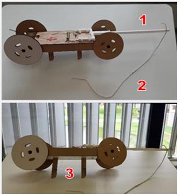
Figure 2. Elements of the mousetrap car: 1. Rod (whose size is defined by the student); 2. String, to connect the rod to the rear wheel axle; 3. Keel, so that it could move around the Track and the sensors could identify its passage
