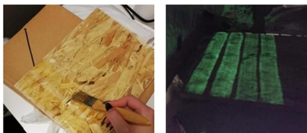
Figure 3 Applying the preparations on the recycled wood boards (left); painting stripes with a different number of layers (right)
