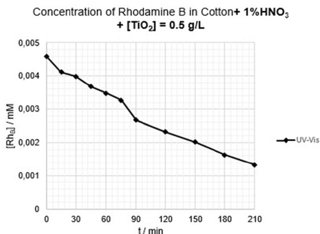
Figure 7. Photocatalytic degradation of RhB using acid-treated cotton coated with [TiO<sub>2</sub>]=0.5 g / L
