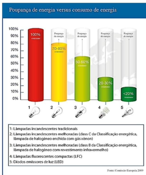
Figure 1. Energy savings versus energy consumption
