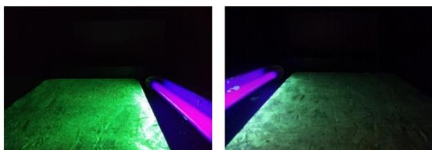
Figure 5. On the left, a wood board painted with the 11,066 g phosphor:10 mL oil solution; on the right, another board, painted with the 11,066 g phosphor:15 ml oil solution, both under “black light”. Brightness is significantly
