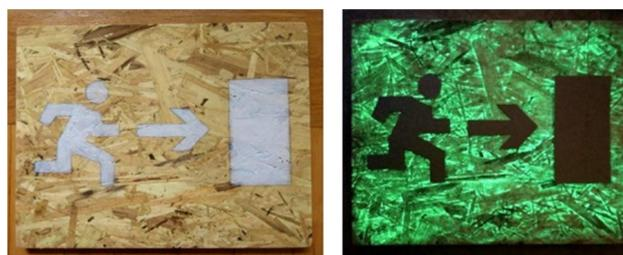
Figure 6. On the left, the finished prototype sunlit, charging; on the right, the same prototype in the dark, glowing, exhibiting the phenomenon of phosphorescence
