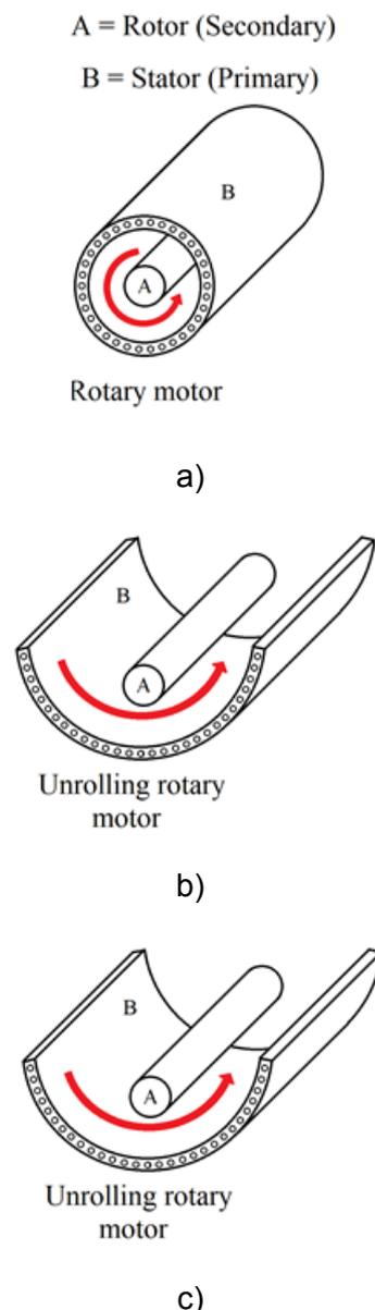
**Figure 5. Rotary motor versus linear motor**
