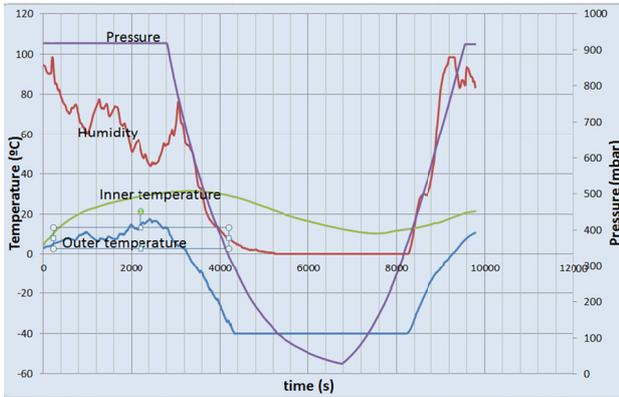
**Figure 17. Time variations of the pressure, inner and outer temperatures, and humidity**
