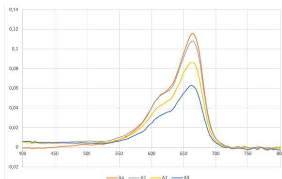
Graph 1. Adsorption spectrum of solutions A0, A1, A2 and A3
