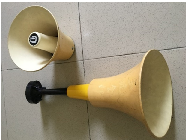
Figure 2. Picture of the horn of megaphone. Horn is separated into three parts and folded
