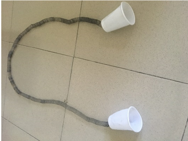
Figure 1. Picture of the echo telephone. Two cups are connected by the long spring
