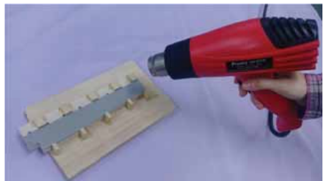
Figure 7. Heat the PVC plate on the mold with a hot air gun. The tool that looks like a hair dryer is a hot air gun
