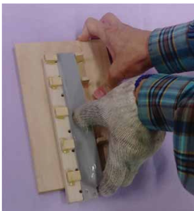
Figure 8. The soften PVC turbine plate is squeezed
