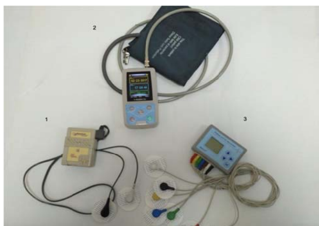
Figure 2. Telemedicine devices: 1 - Heartrak smart (Universal Medical Inc.) event monitoring device; 2 - Heaco blood pressure monitor; 3 - DiaCard 3 channel monitor
