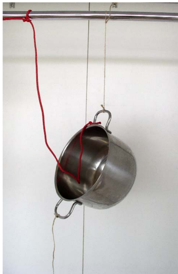
Figure 3. The pot prepared for the breaking of the string (The thicker string acts as a safety device to prevent the pot from striking the floor)
