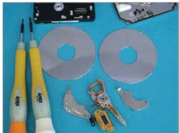
Figure 2. Removed parts from HDD
