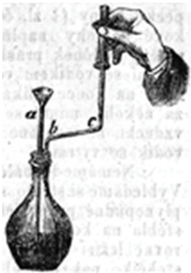
Figure 4. Hydrogen generation apparatus [4]
