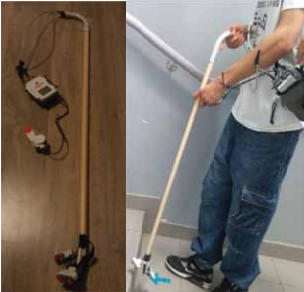
Figure 6. The smart walking stick
