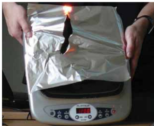
Figure 6. Burning an aluminium foil caused by eddy currents above the plate of heater
