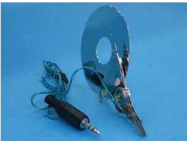
Figure 5. An example of the bone conduction speaker
