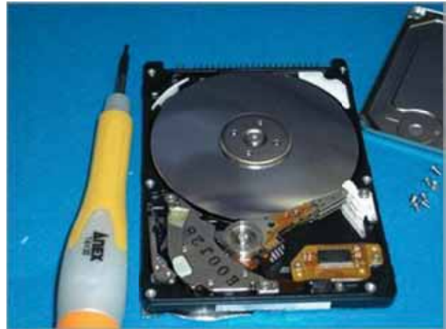
Figure 1. Removed cover from 2.5 inch hard disk drive
