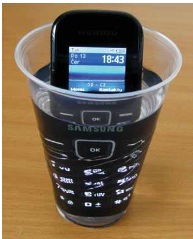
Figure 7. Mobile phone sunk in NOVEC 1230
