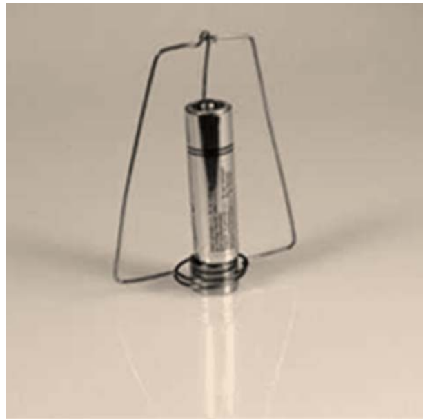
Figure 3. One loop electric motor
