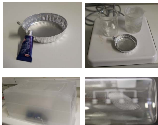
Figure 2. Revealing latent fingerprints using superglue fuming
