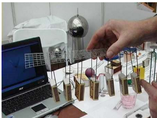
Figure 4. Wave machine made from match boxes
