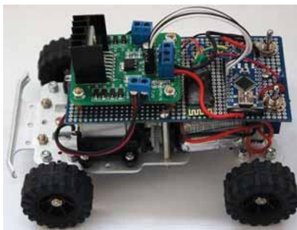
Figure 3. A remote controlled car built with Arduino
