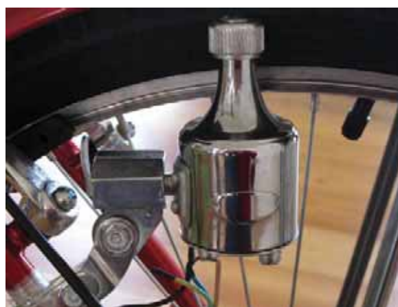
Figure 4. AC voltage generator fitted in the back wheel frame of a bicycle
