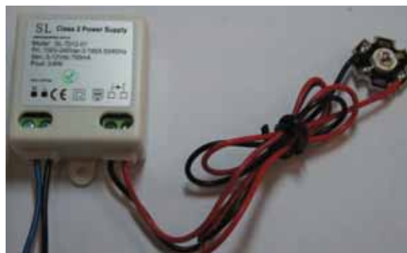
Figure 4. 6 watt commercial power source and power LED
