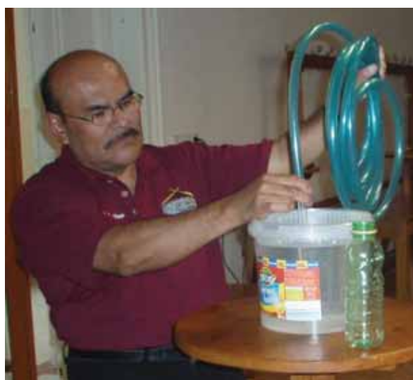
Figure 4. Single-tube apparatus to measure atmospheric pressure
