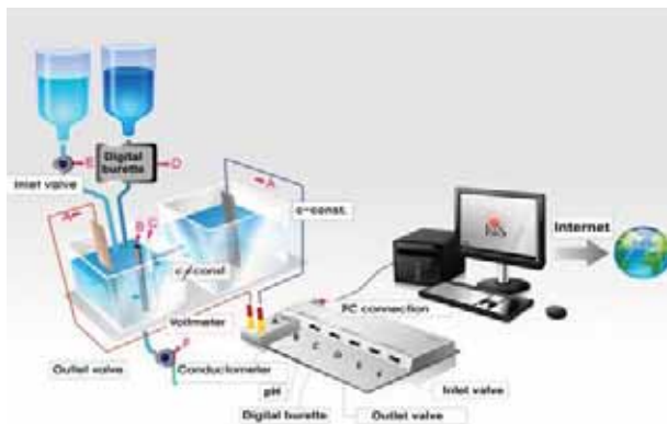
Figure 3. Schematic diagram of the remote interactive experiment Electrochemical cell characterization
