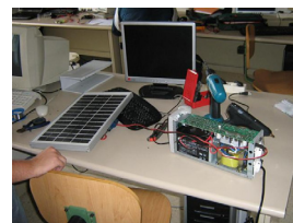
Figure 16. Electrification kit with solar recharged UPS
