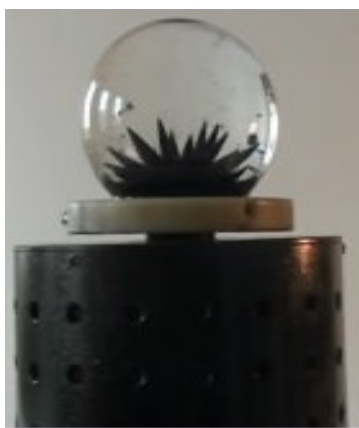
Fig. 4. The magnetic field of electromagnet showed by ferrofluid.
