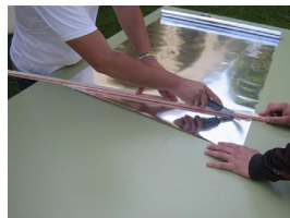
Figure 18. Cutting reflective sheet
