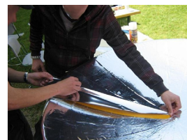
Figure 19. Applying reflective sheet
