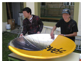
Figure 19. Applying reflective sheet
