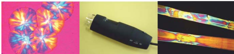
Figure 2. Picture of spherulite crystals of PP (left). Microscope model USB PCE-MM 200, which allows the observation of the previous structure (centre), and view through polarizing sheets of large crystals obtained by stretching of PP sheets (right)
