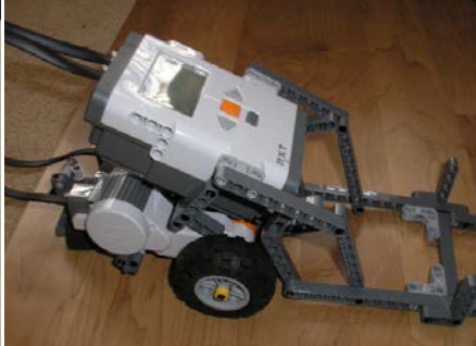
Figure 3. FLL LEGO robot - NXT controller
