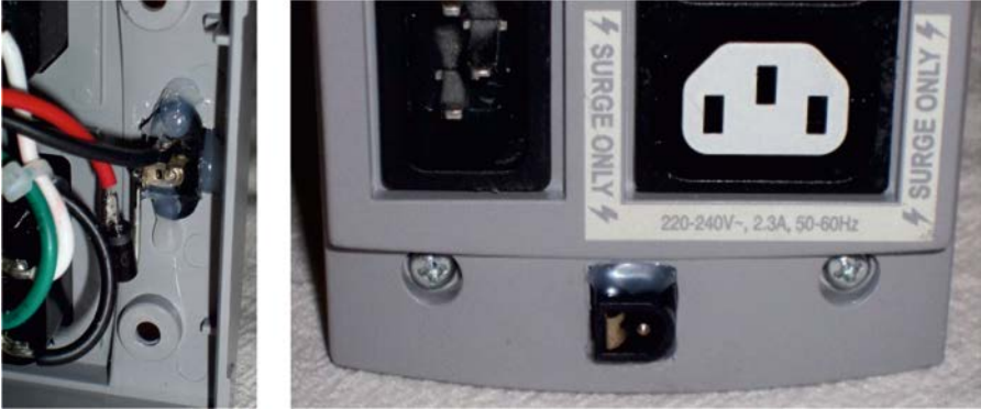
Figure 5. External recharge connector
