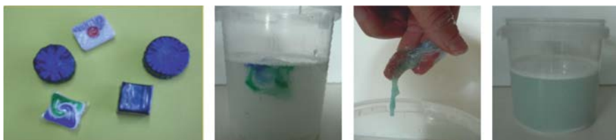
Figure 7. Different type of commercial products covered with plastics soluble in water and illustration of the plastic dissolution when the tablet is immersed in warm water
