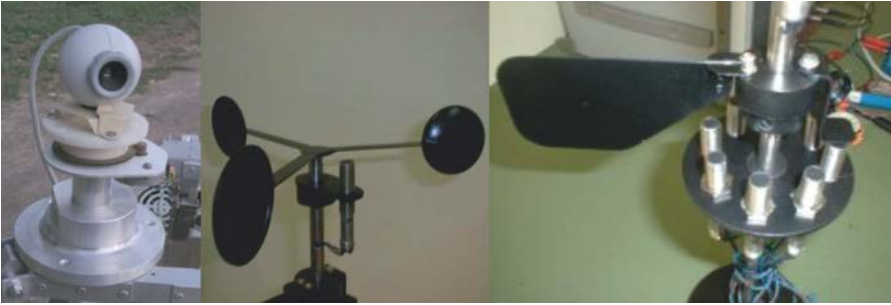
Figure 3. The camera, the cup anemometer and the weathercock
