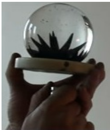
Figure 3. The magnetic field of permanent magnet showed by ferrofluid
