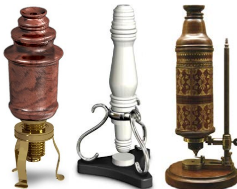
Figure 2. Divini's vase-shaped microscope (left), Campani's ivory turned monocular microscope (centre) and Cock's compound microscope, manufactured in London for R. Hooke (right)
