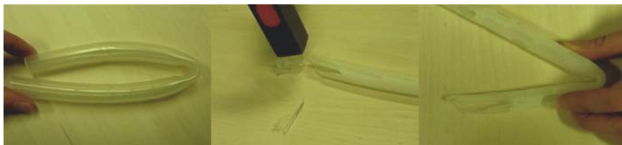
Figure 4. Rubber hose bent at room temperature (left). Brittle behaviour when it is being hit by a hammer, after the introduction into liquid nitrogen (centre). Recovery of the flexible behaviour after a few minutes at room temperature (right)
