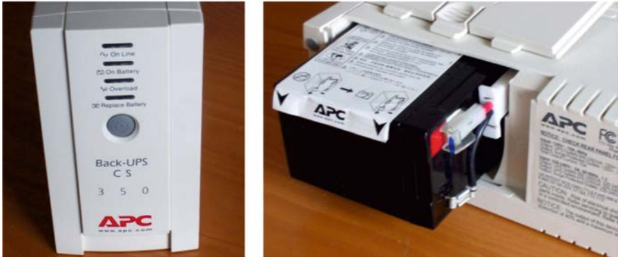
Figure 3. UPS and battery housing
