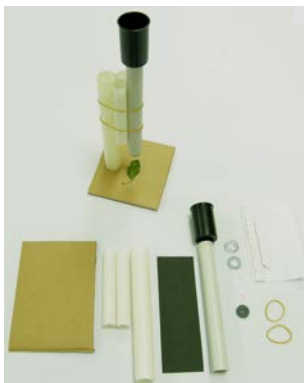
Figure 6. The materials used & the first version of the constructed microscope with 2 lenses
