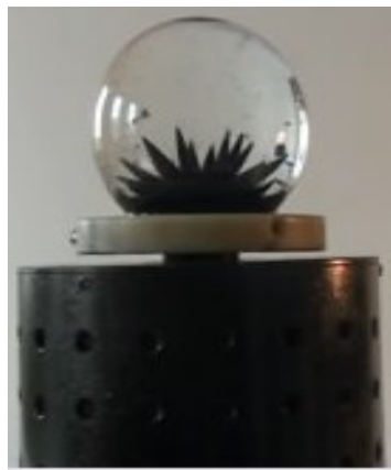
Figure 4. The magnetic field of electromagnet showed by ferrofluid
