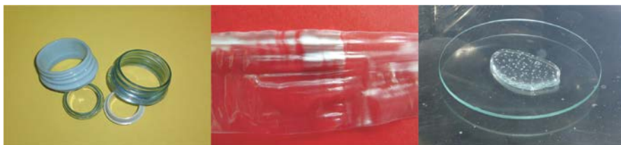
Figure 3. Thread of PET before (transparent) and after the introduction into boiling water (left). Opacity generated in PP when it is stretched (centre). HDPE transparent obtained when it is heated above 140^{\circ}\text{C} (right)
