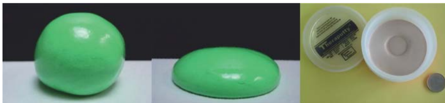
Figure 5. Illustration of the viscous behaviour of the Silly Putty®: ball (left) that is spilled on a flat surface (centre) and disappearance of the bas-relief of a coin with time (right).
