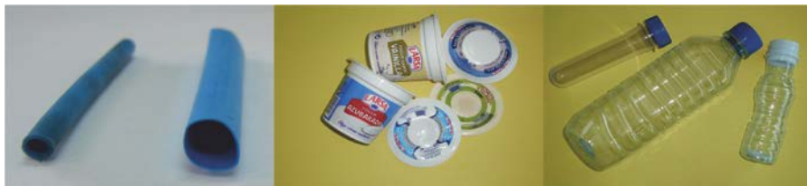
Figure 6. Shrink PE before and after submitting to heat source (left). Recovering of the original shape (a sheet) of yogurt glass made with PS (centre). Tendency to recover the original shape (cylinders or perform) of PET bottles (right)
