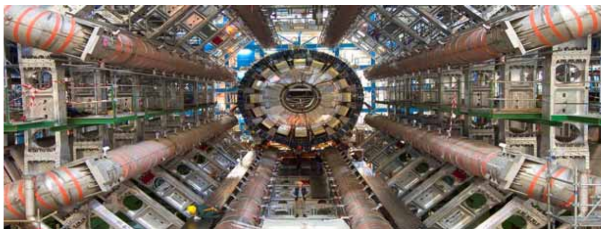
Figure 5. The ATLAS detector under construction at CERN. The man at the bottom of the photo indicates the scale of the detector
