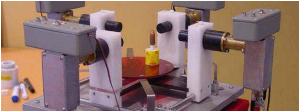
Figure 2. A simple PET camera. Each pair of movable detectors is coupled in coincidence. During the demonstrations the source is covered
