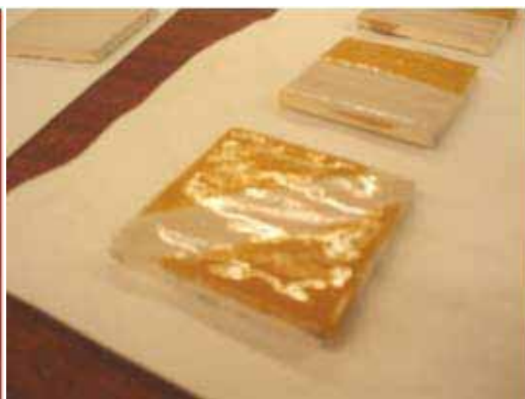
Figure 2. Azulejo produced by cold processing using polymer cross-linking
