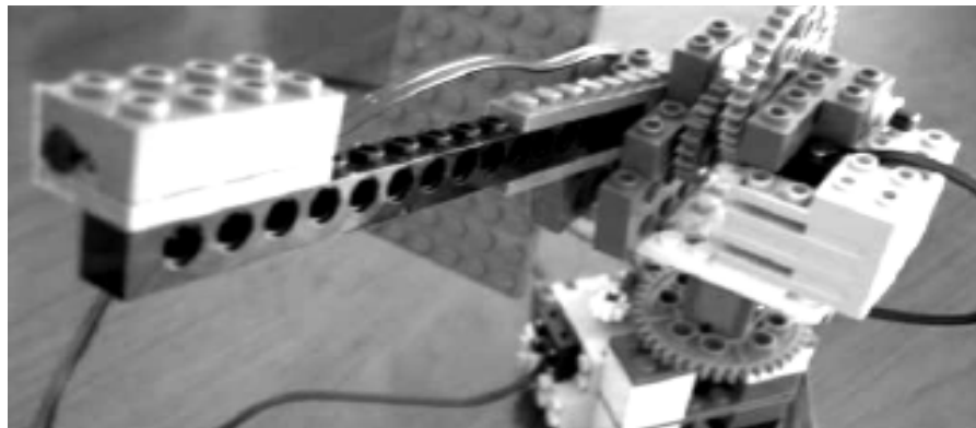
Figure 3. Two-axis orientation system
