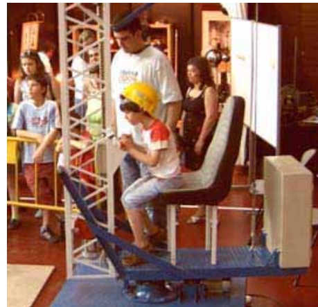
Figure 4. Operating the crane via the control panel (the switchboard is behind the operator's seat)
