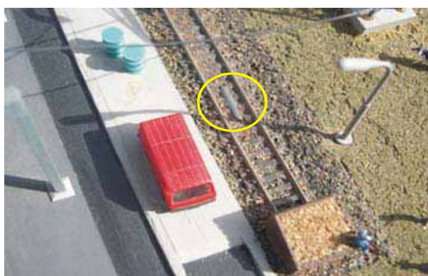
Figure 15. Reed relay placed between the rails
