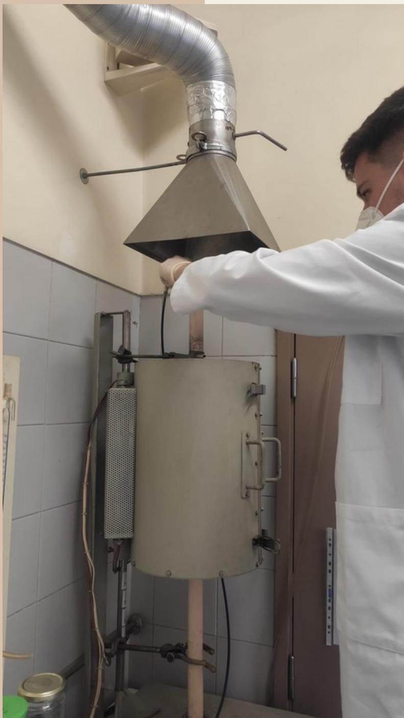
Fig. 14 - Placing the basket in the pyrolytic reactor(14)
