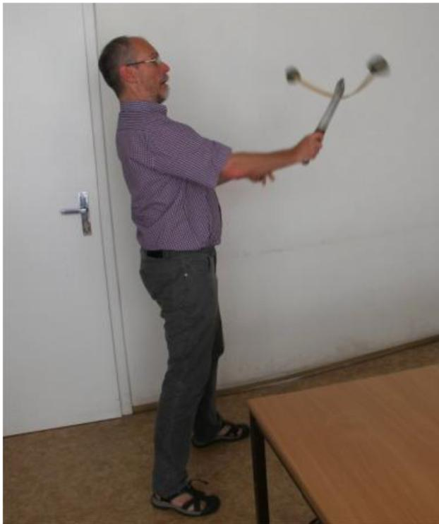
**Figure 5. Breaking the flying bar is easier after loading its ends with plasticine**
