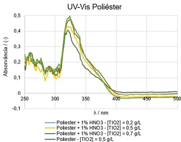
Figure 4. DRUV-Vis characterization of polyester substrates
