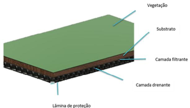
**Figure 1. Technical design of an extensive green roof**
