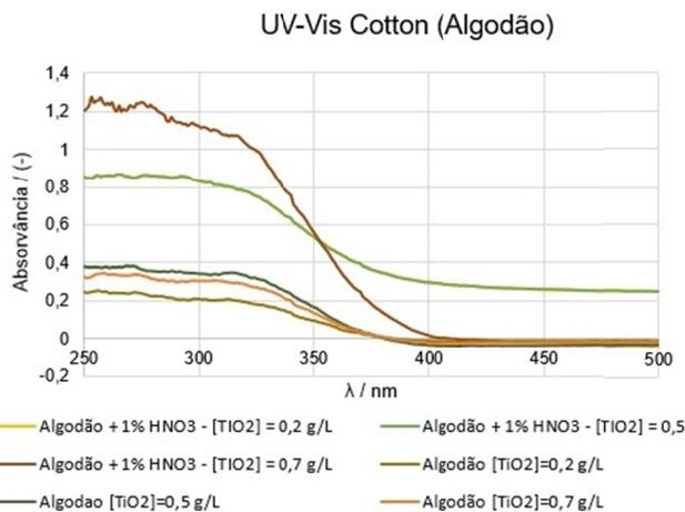
Figure 3. DRUV-Vis characterization of cotton substrates
