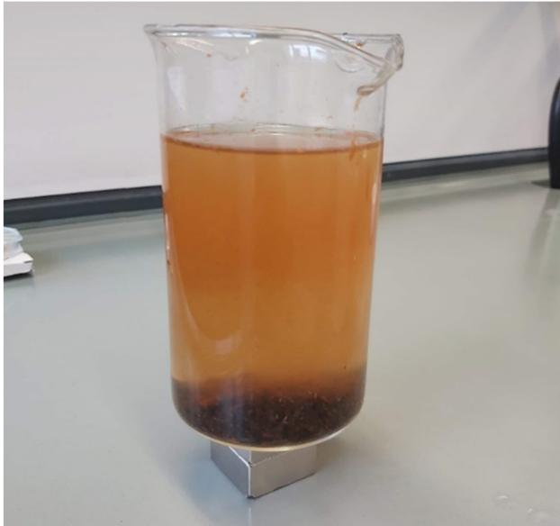
Figure 1. Interaction between nanoparticles and magnet
