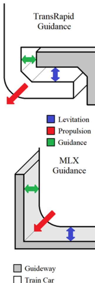
Figure 3. Levitation, propulsion, and guidance in MagLev
