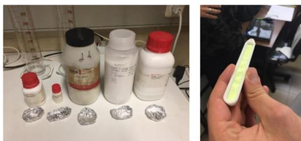
Figure 4. On the left, the reagents used in the production of  $\text{SrAl}_2\text{O}_4: \text{Eu}, \text{Dy}$ ; on the right, the already produced phosphor
