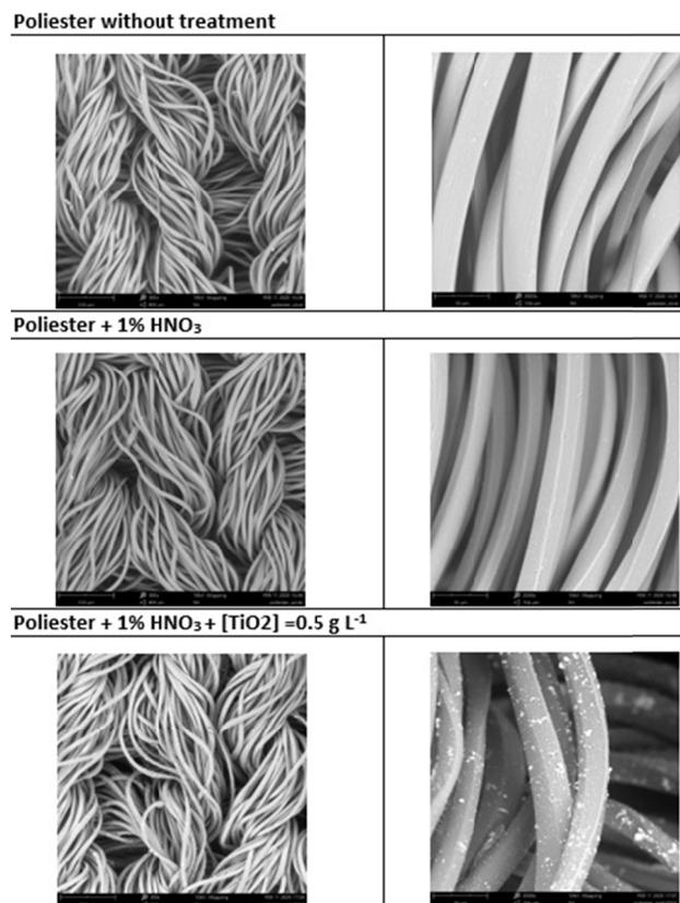
Figure 6. SEM characterization of polyester substrates
