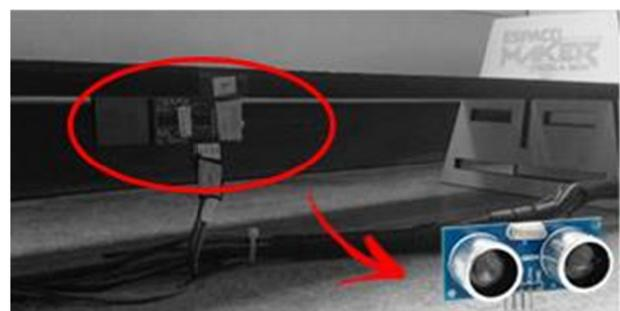
Figure 6. Highlight: sensor that starts the stopwatch
