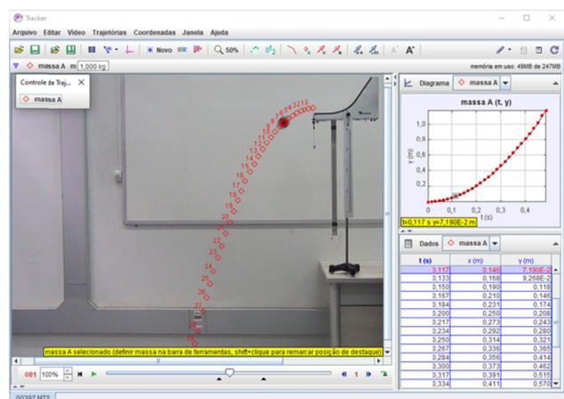
Figure 3. Print of the software Tracker screen of ball thrown horizontally
