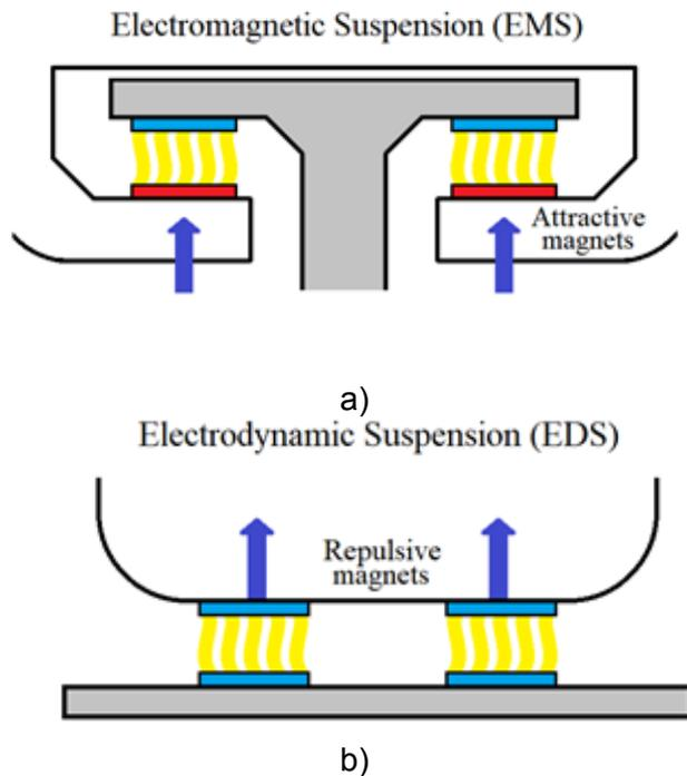
**Figure 4. Electromagnetic suspension (uses attractive magnetic forces) (a) and electrodynamic suspension (uses repulsive magnetic forces) (b)**
