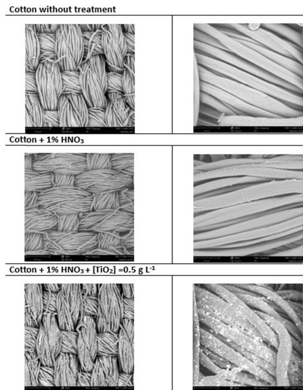
Figure 5. SEM characterization of cotton substrates
