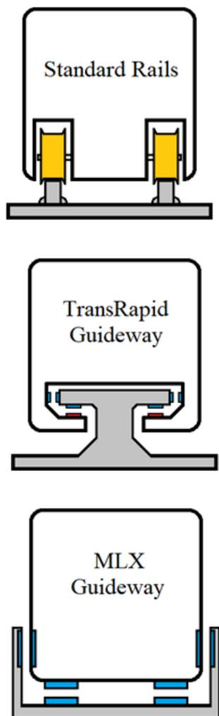
Figure 2. Comparison of Wheel-Rail versus Guideways
