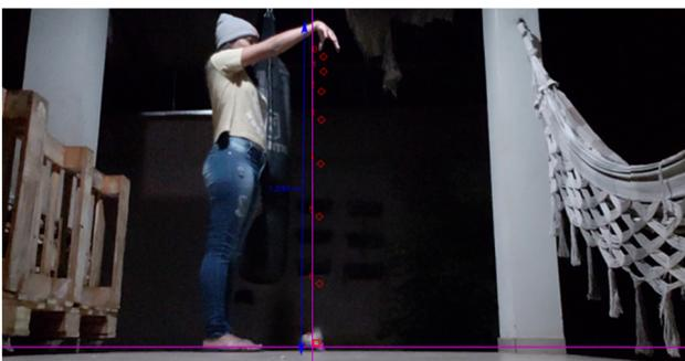
Figure 5. Analysis of an object in freefall
