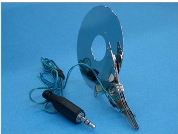
Figure 5. An example of the bone conduction speaker
