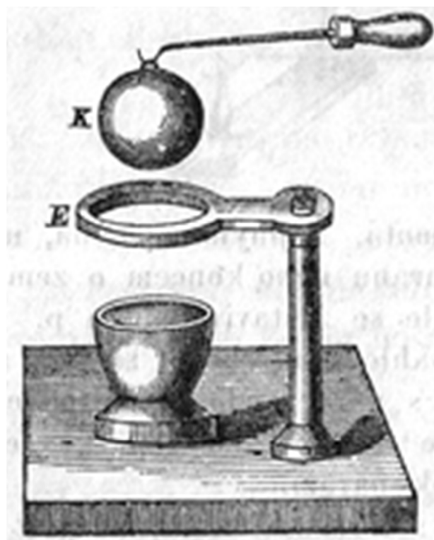
Figure 3. Thermal expansion of metals [9]
