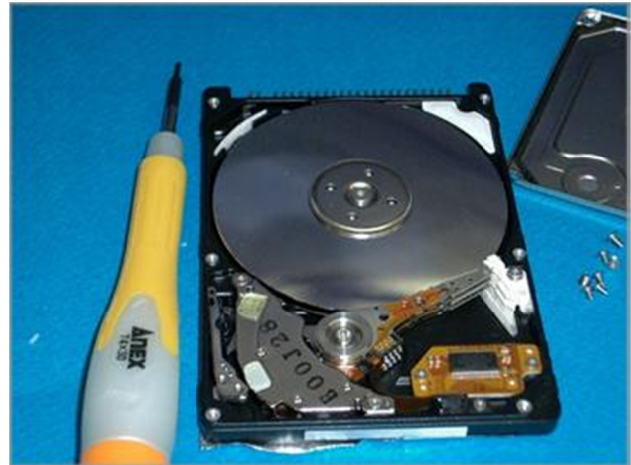
Figure 1. Removed cover from 2.5 inch hard disk drive
