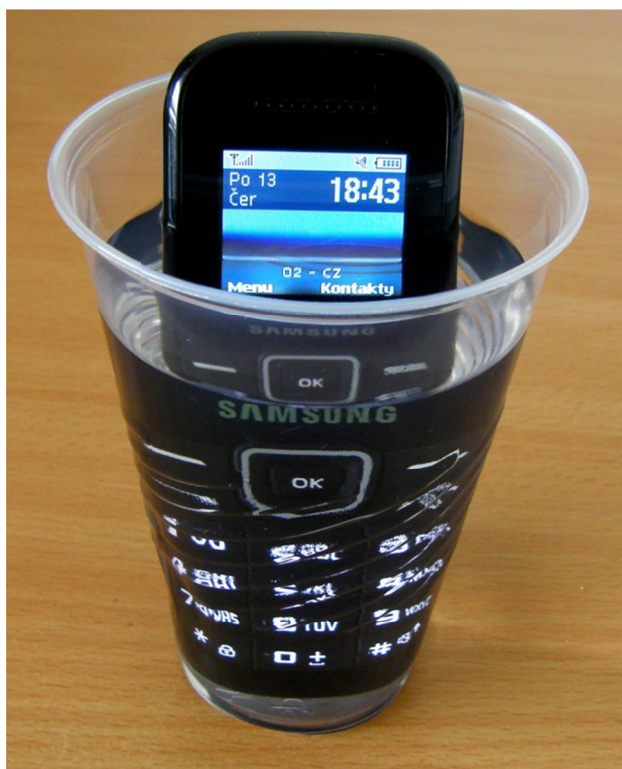
Figure 7. Mobile phone sunk in NOVEC 1230
