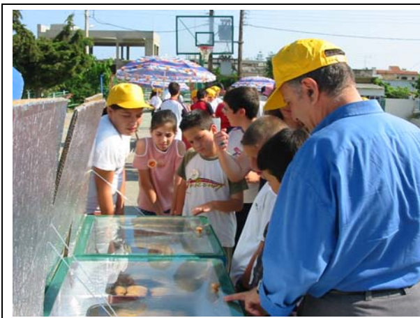
Photo 5: Box solar cookers, as presented in the science fair, cooking biscuits and cakes for children and visitors to taste in temperatures ranging from 110 to 120 °C.
