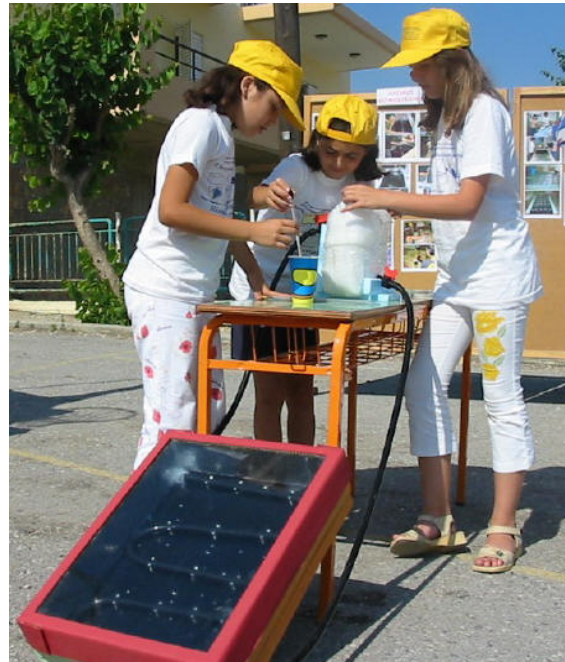
Photo 4: Final presentation of the “serpentine solar heater” in the science fair, with an improved incline for the serpentine loops, an improved water tank and some coloring.
