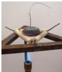
Fig7: Quantitative oxidation of magnesium
